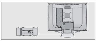
1 Connect the white and red sockets »AUDIO OUT L R « on the television and the corresponding sockets on the HiFi with a cinch cable.
